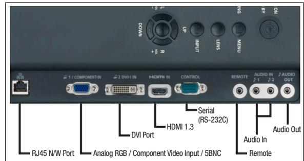
Expanded interface options include DVI-I, HDMI 1.3, and analog RGB inputs. Control connections include a network-ready RJ-45 port and RS-232C serial connection. A separate stereo mini-jack input enables direct connection with the hand-held remote-control, if desired.
