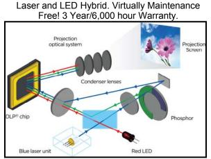
By combining a laser, a fluorescent element and an LED Casio has created an original mercury-free hybrid light source capable of generating high brightness. Casio has achieved high brightness output of green light, which until now, has been considered difficult with conventional semiconductor light sources, by efficiently converting blue laser light into green light using a fluorescent element.
