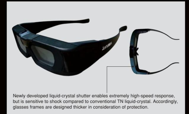
Newly developed liquid-crystal shutter enables extremely high-speed response, but is sensitive to shock compared to conventional TN liquid-crystal. Accordingly, glasses frames are designed thicker in consideration of protection.
