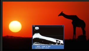
The PT-AE2000 gives home consumers a projector with the kind of waveform monitor used in equipment for professionals.
