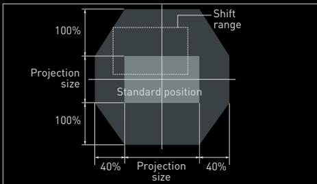
to project a 120-inch picture from as close as 11'10" (3.6 m) to the screen or as far as 23'7" (7.2 m) away. In addition, the image can be shifted  $\pm 100\%$  vertically, and  $\pm 40\%$  horizontally. This gives you outstanding setup flexibility. If you choose to ceiling-mount the projector, you can zoom and focus by remote control.
