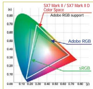
Proprietary color filters incorporated into the AISYS optical system deliver exceptional accuracy and detail in both Adobe RGB and sRGB modes. This is ideal for professional photography, design, publishing, printing and fine art, where color integrity is crucial.
