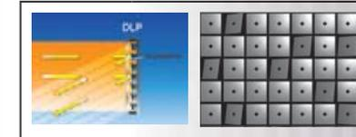
A constantly rotating color wheel reflects red, green, blue, and white image components off a micro-mirror device to produce the projected image. The three primary colors are sequentially displayed and synthesized in the viewer's brain to produce images perceived as full color.
