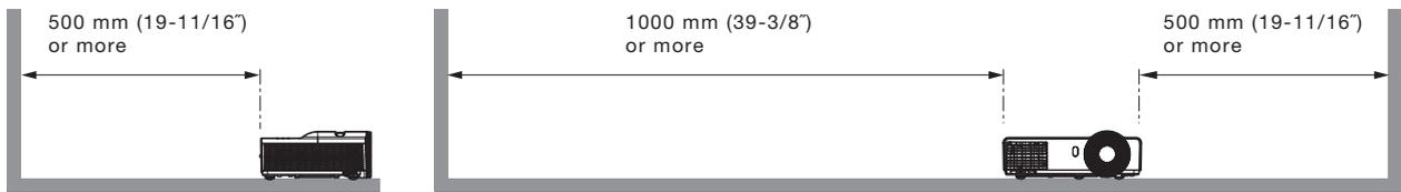
**Direction of air intake and exhaust**
